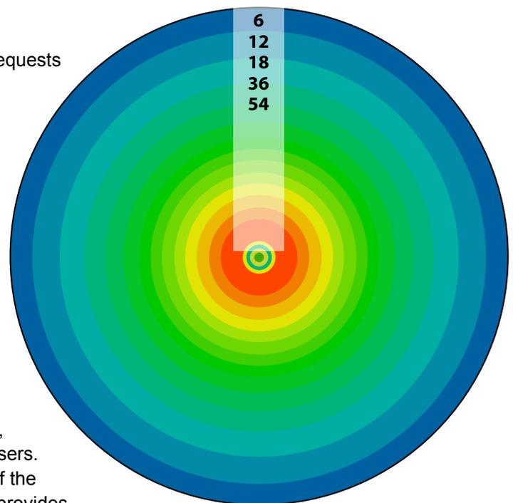
**Figure 1: Modulation rates decline as users move away from the Wi-Fi AP**
