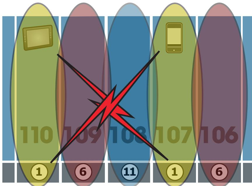
Figure 4. AP to non served client devices or client device to non serving AP interactions
